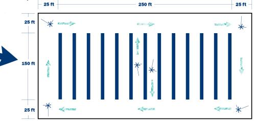
The diagram shows six Herkules 7 ft vertical, tri-pole mount ceiling fans working together to create facility-wide air flow that isolated, downward facing fans cannot match.
